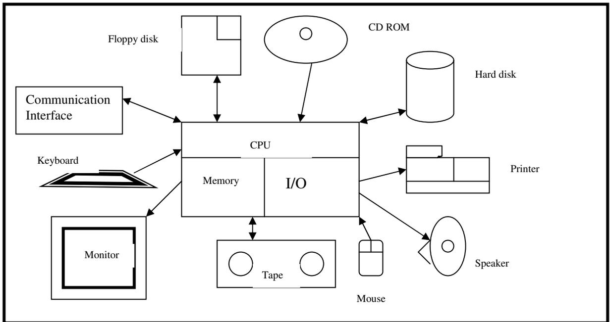
Fig.3.2 A typical Computer System
